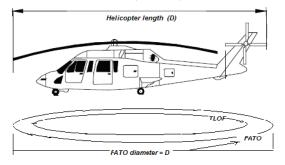
A FATO is an area over which a helicopter completes the approach manoeuvre to a hover for landing or commences movement into forward flight in the take-off manoeuvre. A FATO may be any shape but must meet the requirements of 139.I.21(d)2 which states
