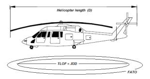
Whenever it is intended that the undercarriage of a helicopter will actually touch down on the surface of a heliport or leave the surface to achieve a hover, a touchdown and lift-off area shall be provided. The dimension of the area shall be of sufficient size to contain a circle of diameter 0.83D of the largest helicopter the area is intended to serve and be dynamic load bearing when located within the FATO.
