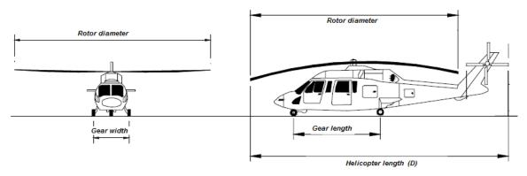
Critical aircraft considerations for a fixed wing aerodrome include runway operational length, aircraft width and undercarriage width to code aerodrome in accordance with OTAR 139.B.05.
